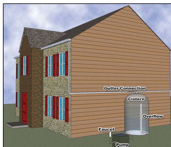
Figure 7.42: Major Components of a Rainwater Harvesting System
